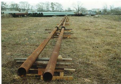
Test loop designed for evaluation of different thick film coating material for application to heavily pitted pipeline.
